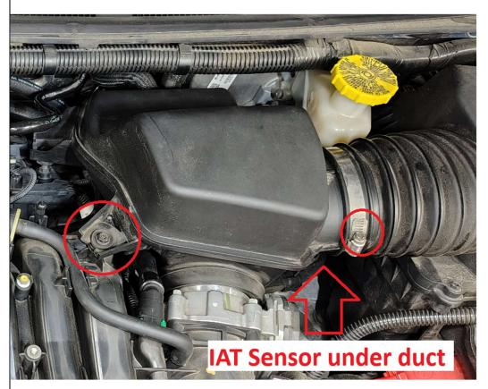
Slide duct with clamp off air box, lift rear of airbox off of rubber grommet. Then push the airbox off the throttle body, there is no clamp here. Pull air box past throttle body.
