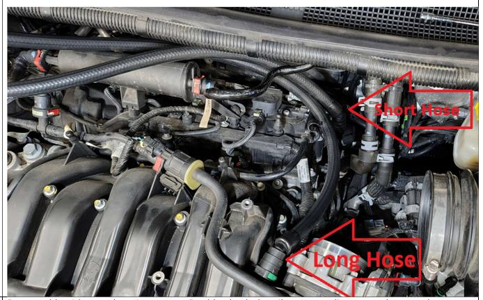
**9** Reassemble airbox and engine cover. Double check the oil separator lines to make sure they are not pinched; the long line should route under the airbox.
