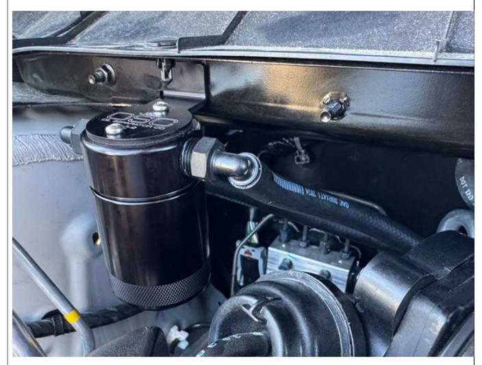
7 This completes your installation. Average collection on most vehicles is roughly an ounce of oil every 1000 Miles, the can holds 3 ounces. In cold climates expect condensation to mix in the can in the winter months, which will fill it faster.
