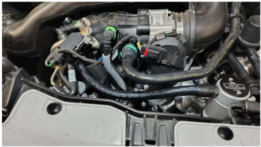
If you ever need to remove these fittings in the future, press the larger portion of the green clip inward to release. It's a button! Don't remove the clips!
