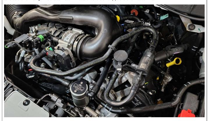
The long hose with the straight fitting will install onto the valve cover connection. Route hose as shown in photos below. The fitting will produce a slight audible "click" when engaged.
