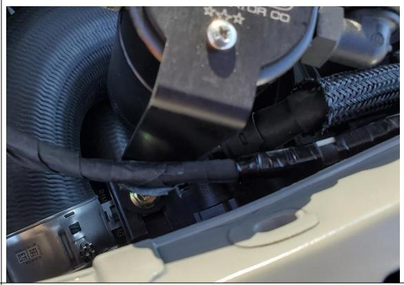
The hose with the straight fitting will install onto the valve cover connection. Route hose under wiring harness and under the two plastic corrugated lines to make connection at the valve cover. The fitting will produce a slight audible "click" when engaged.
