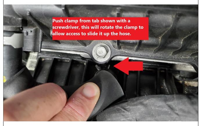
Once the clamp is slid up the hose, you will need to use the flat head screwdriver to get this hose loose. Put the tip of the screwdriver between the end of the hose and the intake manifold. Gently pry up on the hose while pulling up on it to release, it will be TIGHT!
