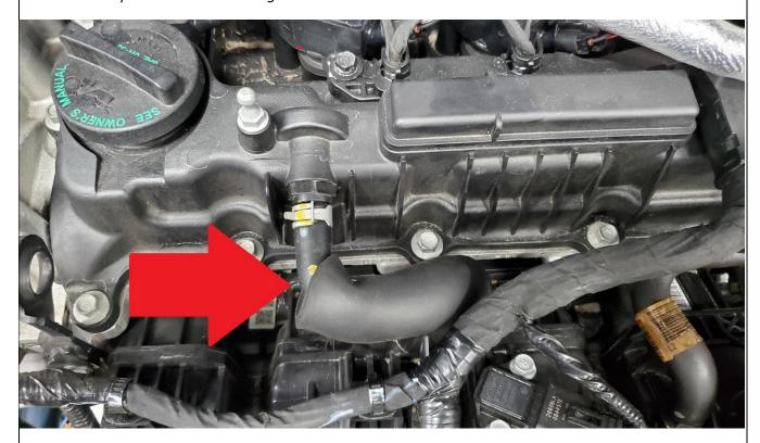
Slide clamp at valve cover back on hose, use pliers to twist hose and while pulling to release it from the valve cover.
