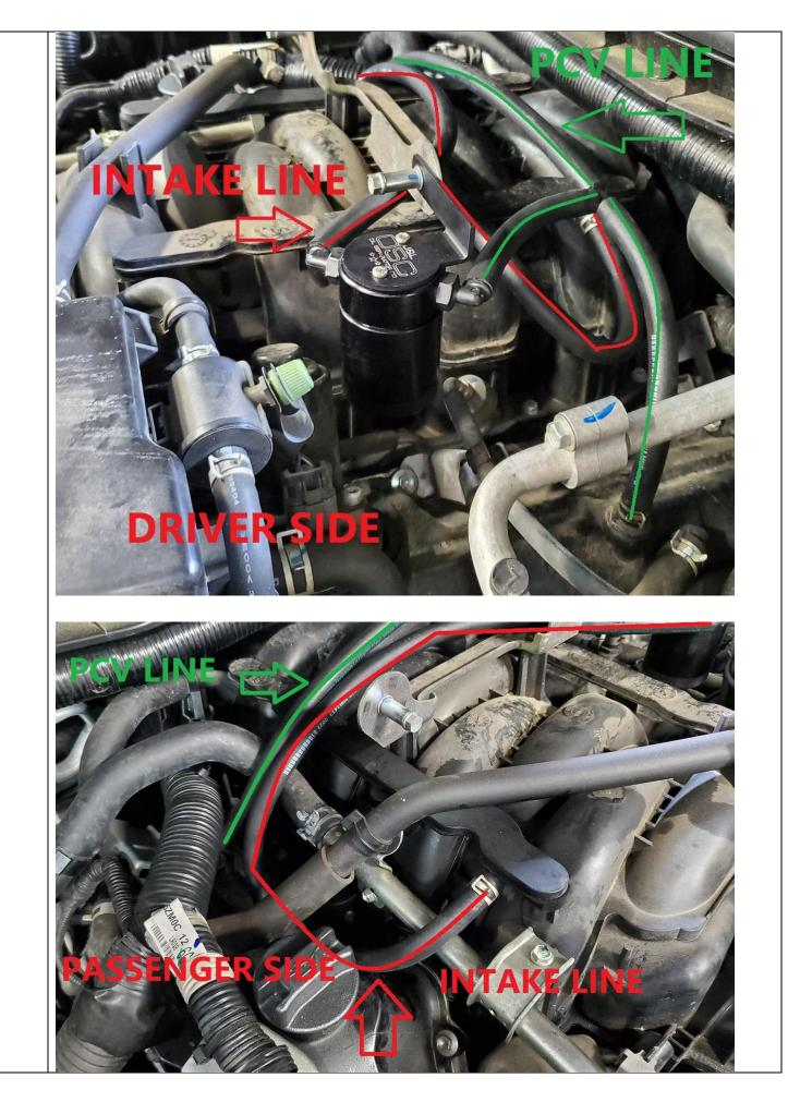
7 Reinstall engine cover. Check oil separator after 1000 miles of driving to gauge how often you will need to service it. The oil separator can be serviced without removing the engine cover, but we do suggest removing it to avoid spills!
