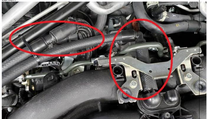
Connect hose that connected to the PCV hose to the "O" side of the J&L Oil Separator. Be sure to install the dress up end on the end of the hose first. Use the same grease to lube end of hose prior to install.
