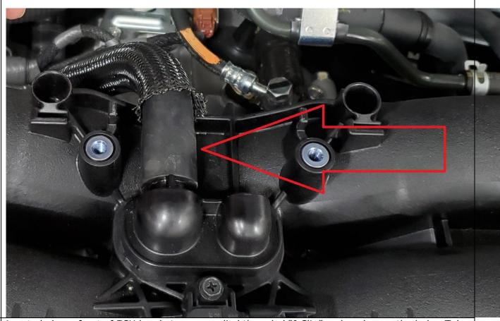
Locate hole on front of ECU bracket, use supplied threaded "J Clip" and push over the hole. Take supplied bolt, washer and J&L Bracket and install bracket into place. Once complete mount J&L Oil separator to mounting bracket with the supplied screws.
