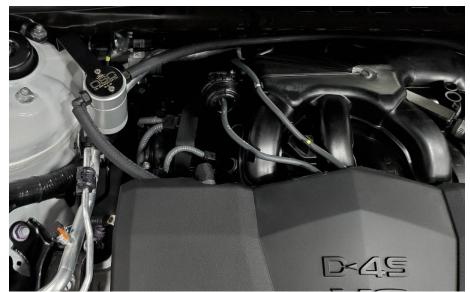
To properly clean the filter in the Oil Separator, spray any degreaser or solvent through it and let it air dry. Clean it every 10,000 miles.
