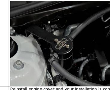
**9** Reinstall engine cover and your installation is complete! Average oil collection is about 1 ounce per 1000 miles, but every engine/vehicle/driver is different. Check oil separator after 1000 miles to get an idea of how much yours is collecting.
