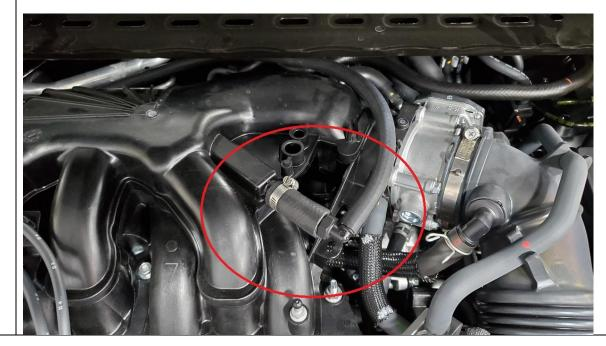
8 Grease or oil inside the hose ends, this will help you slide the hoses onto the oil separator fittings. Check clearance against Air condition line, adjust bracket as needed and tighten mounting nut & bolt.
