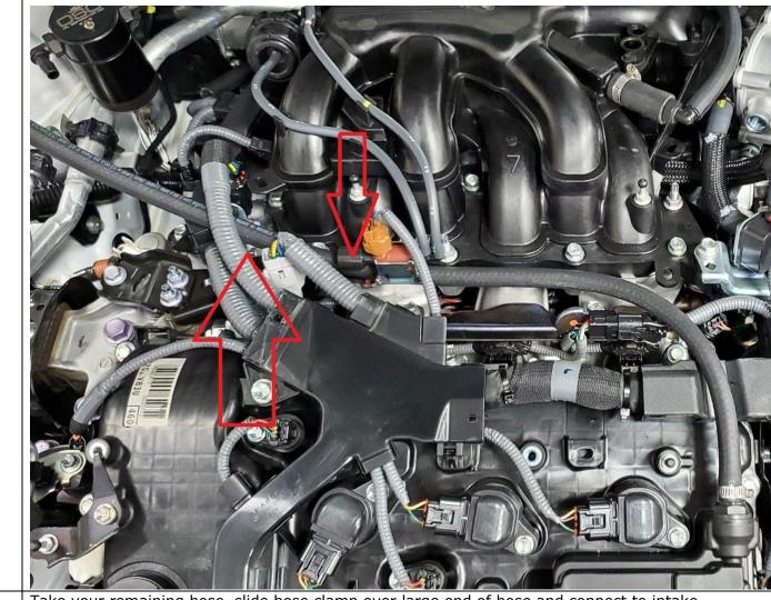
7 Take your remaining hose, slide hose clamp over large end of hose and connect to intake manifold. Route hose around back of intake manifold towards the oil separator. Tighten hose clamp.
