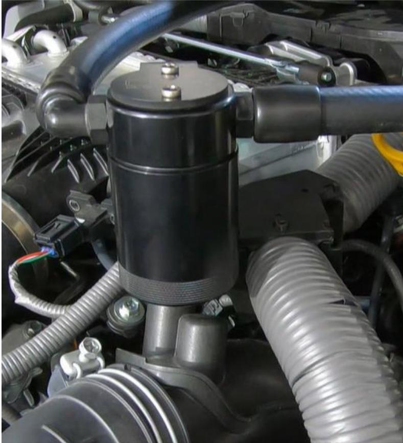
**8** Reinstall engine cover, slide cover into place under J&L hose. The cover attaches to the horizontal bar and into two separate grommets. Be sure cover clears oil separator bracket, you will need to now tighten the bracket bolt. The cover will need to be shifted back out of the way to tighten this bolt.
