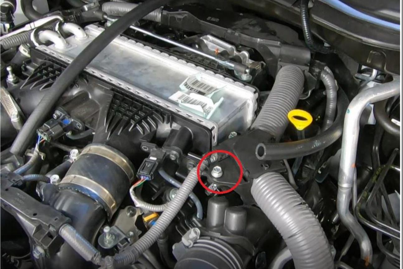
Mount J&L Oil Separator to mounting bracket with supplied screws.
