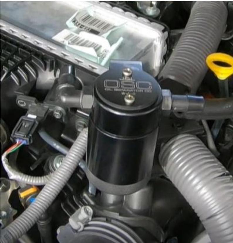
**7** Connect hoses to oil separator, use light grease or oil inside of the end of the hoses (a Q-Tip is useful here). Be sure to slide the dress up ends onto the hose ends before installing hoses onto the oil separator. The hoses should bottom out to the base of the fittings!
