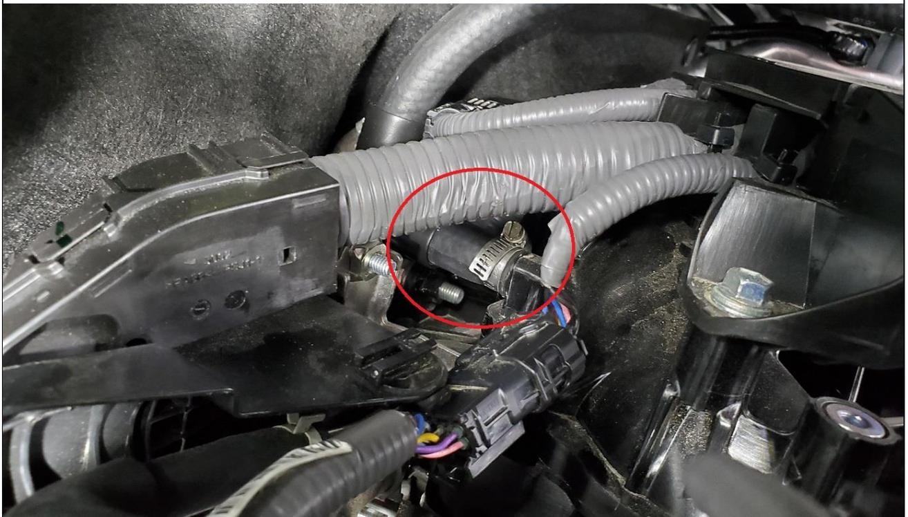
Reattached wiring harness to support.
