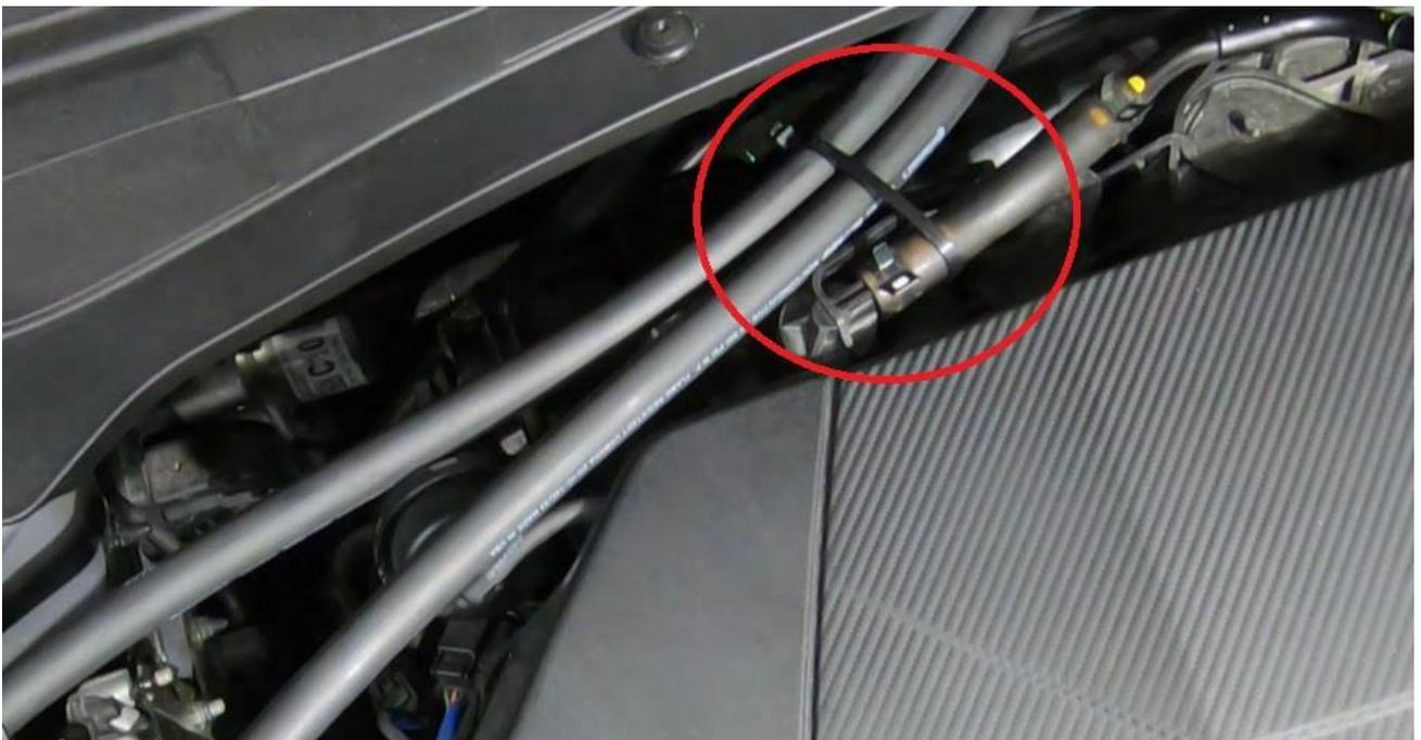
**10** Reinstall the hose bracket and breather line you disconnected earlier in your installation. This completes your installation.
