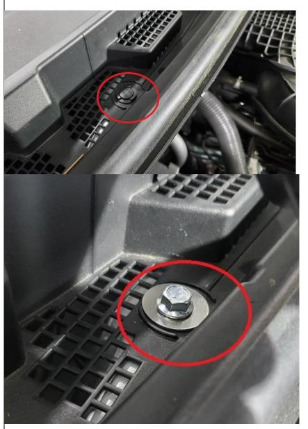
Now take J&L mounting bracket and slide it over the bolt that came through the bottom of the cowl. Use supplied nut to secure bracket but do not tighten bolt completely yet
