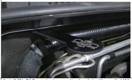
Install J&L Oil Separator to mounting bracket with supplied M4 screws.
