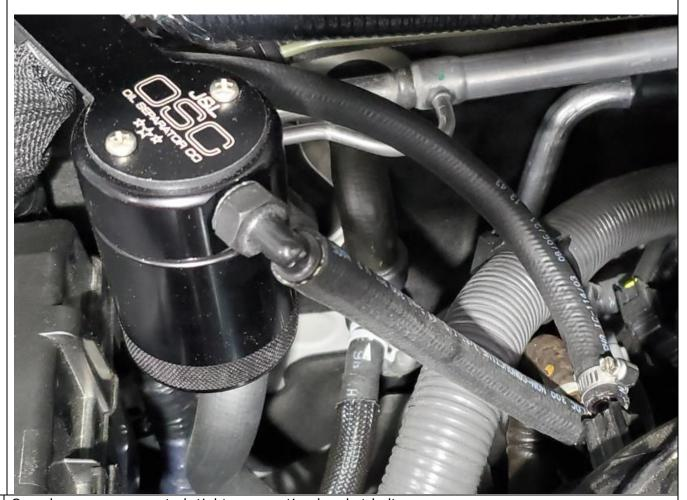
**6** Once hoses are connected, tighten mounting bracket bolt.
