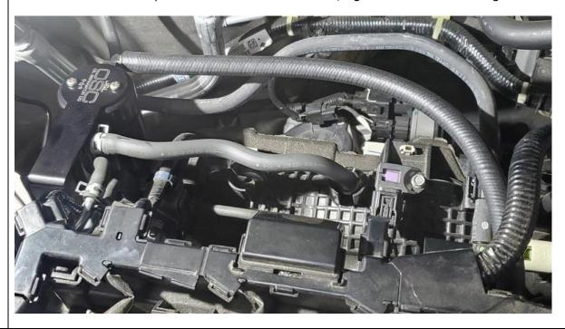
There are two small vacuum lines next to the oil separator, you'll want to rotate the clamp 180 degrees to get it away from the small wiring harness near it. Use the supplied Zip tie to secure black and white harness to small vacuum line. The Zip tie doesn't need to be very tight, just enough to secure it to avoid abrasion from the sharp clamp and bracket.
