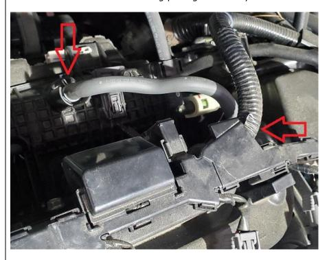
We are going to reuse this hose to connect to the oil separator. You will "flip" the hose, the portion that was connected to the valve cover is going to connect to the intake manifold and run towards the oil separator location. Install hose but do not slide clamp into place yet.
