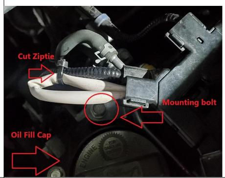
Locate PCV hose, it connects from the valve cover to the intake manifold. Squeeze clamps with your needle nose pliers and slide up hose. Using the same pliers twist hose where it connects to break "seal" twist hose whiling pulling hose away from connection to remove.
