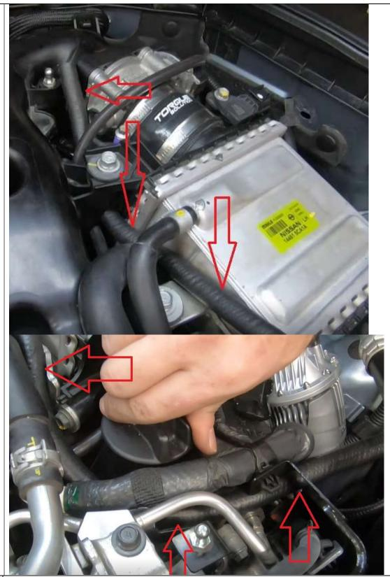
Shorter hose – This hose will route from the oil separator to the PCV valve connection.
