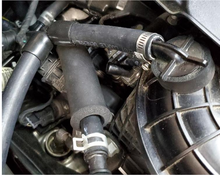
Once the hoses are in their ideal location, tighten the 12mm bolt to secure the J&L assembly.
