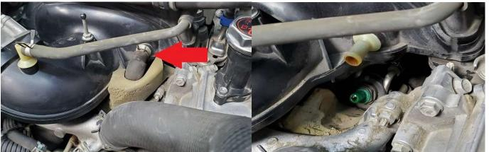
**Hose prep** – Install the factory smaller spring clamp onto smaller J&L line. Pre-grease inside of J&L hoses, this will help with pushing hoses onto factory fittings.
