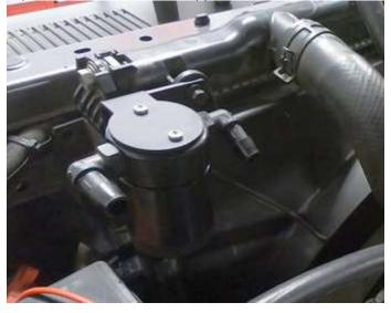
**Note:** 2021 Owners will need to use the supplied J&L Bolt and spacer between the radiator shroud and J&L bracket.
