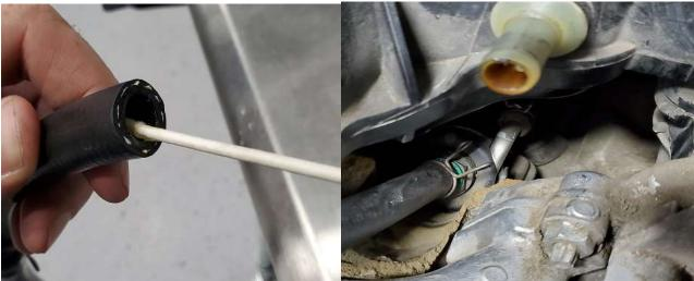
5 Slide the clamp supplied by J&L over the other J&L hose and install onto intake manifold fitting.
