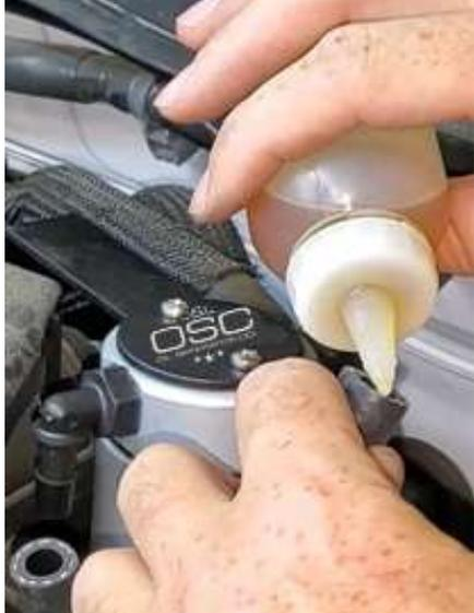
Using light oil, lube the inside of the hoses or can fittings. This will help install the hoses onto the can, no clamps are needed. The hose from the valve cover will install onto the "C" side of the can (OSC). The hose from the intake manifold will install onto the "O" side of the can.
