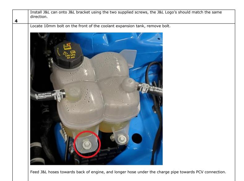
Install J&L Assembly using J&L supplied bolt. **Do not fully tighten bolt yet.**
