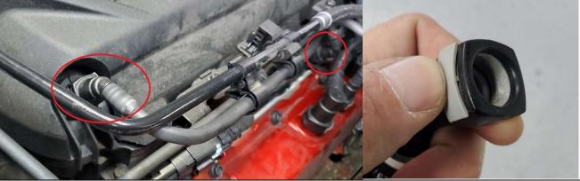
Use the supplied screws and attach J&L Separator to the bracket. Line up the J&L logos.
