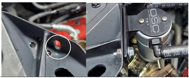
Use your light oil to lubricate the factory fittings on the intake manifold and PCV, this will help to ensure the J&L fitting's slide easily onto them to ensure the O-rings stay in place. We recommend putting a small amount of oil on your finger and applying it to the fittings that way.
