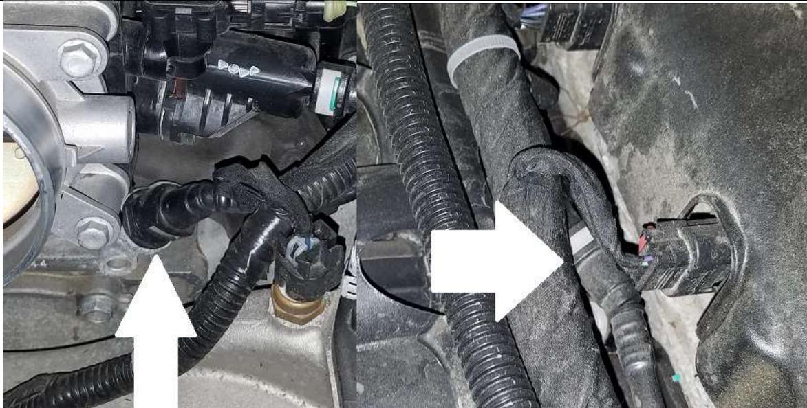
**6.2L Models.** The PCV line is on the front of the engine, seen below. Depress grey tabs to release hose.
