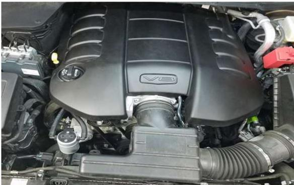
To properly clean the filter in the Oil Separator, spray any degreaser or solvent through it and let it air dry. Clean it every 10,000 miles.
