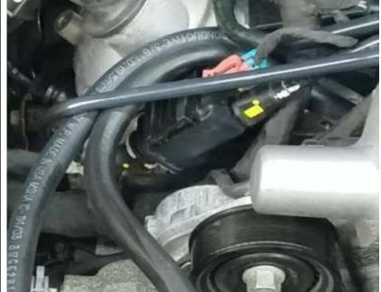
7 The hose from the intake manifold will run to the O (OSC) side of the can, the hose from the valley cover (dirty side) will run to the C (OSC) side of the can.
