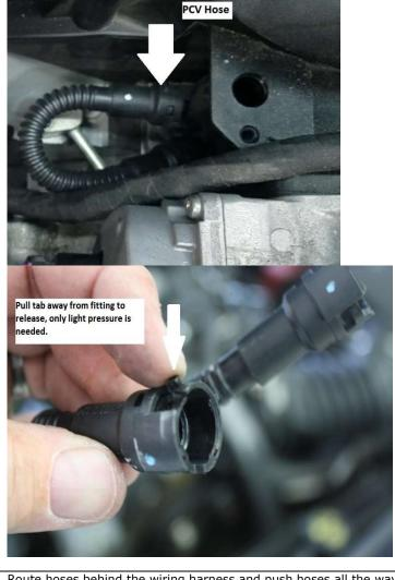
Route hoses behind the wiring harness and push hoses all the way to the barbs on the engine fittings, you will hear/feel a click as they engage. Route hoses between the EVAP solenoid and EVAP hose.
