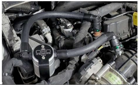
Connect the two hoses to their appropriate fittings. **TIP:** The quick connect fittings at the end of the hose will rotate 360 degrees for adjustment, they may be tough to break free initially, but they will move!
