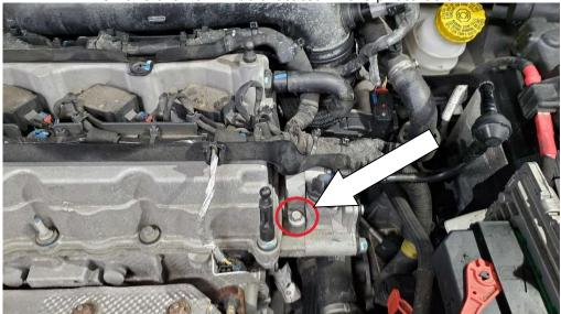
Mount J&L Oil Separator assembly to this location with the same bolt you removed.
