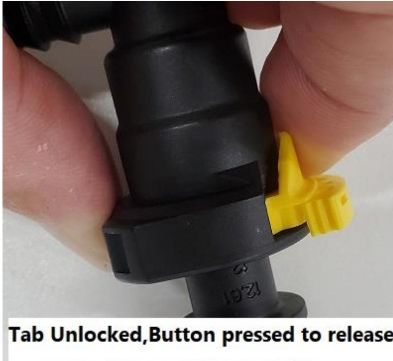
**TIP:** The quick connections are all adjustable in the end of the hoses, if the fitting isn't at an optimum angle, twist the fitting until it is. The hoses can also twist on the J&L Oil separator connections for adjustment, use the natural bend of the hoses to your advantage.
