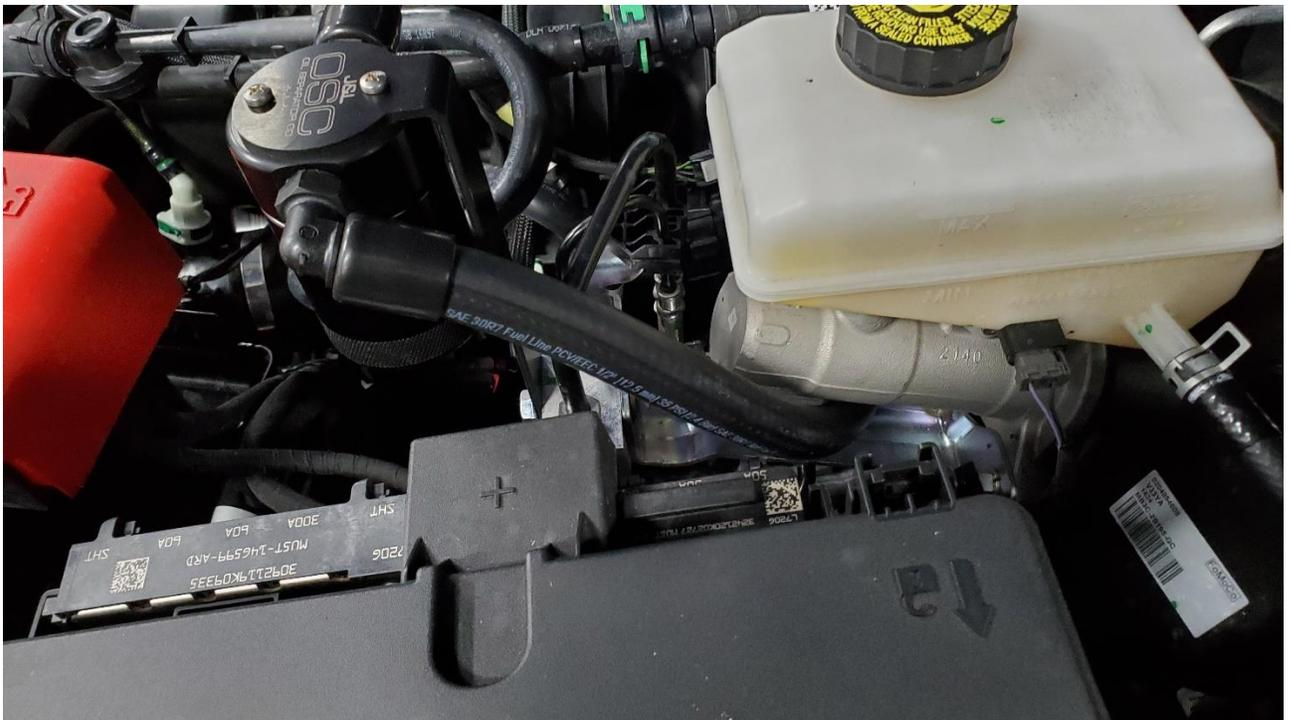
Connect hoses to the valve cover and to the factory PCV line.
