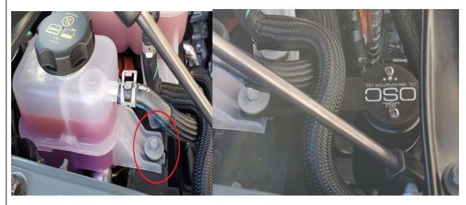
Page 1 of 2 1-27-23 The shorter hose will connect to the PCV valve on the valve cover.
