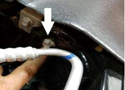
Mount J&L Oil separator to bracket with supplied screws, the fittings should be facing the driver side of the truck.
