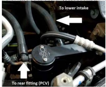
Once hoses are installed. Use supplied zip ties to keep hoses together and neat.
