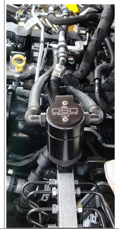
8 Check oil separator after 1000 miles of driving to gauge how often it needs to be emptied. Every vehicle is different!
