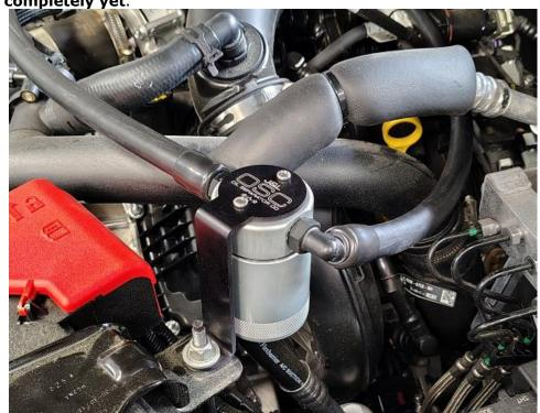
Connect the hose from the "O" side of the oil separator to the PCV fitting on the valve cover. This hose can rest on the rubber isolator that is holding down the two silver coolant pipes.
