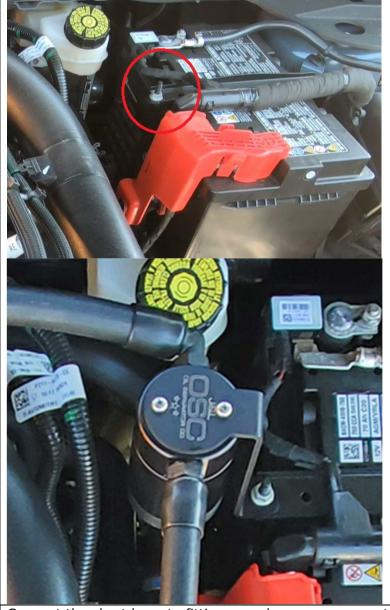
7 Connect the short hose to fitting on valve cover, connect the long hose down to the intake manifold.
