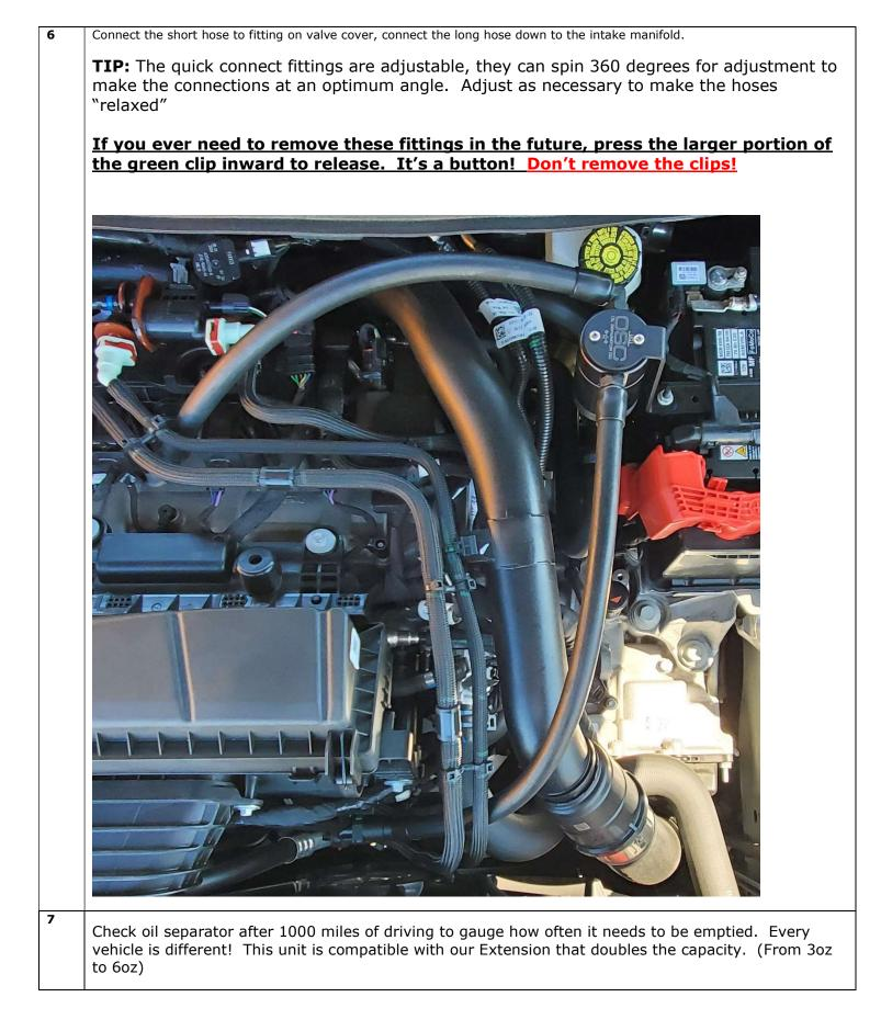
To properly clean the filter in the Oil Separator, spray any degreaser or solvent through it and let it air dry. Clean it every 10,000 miles.
