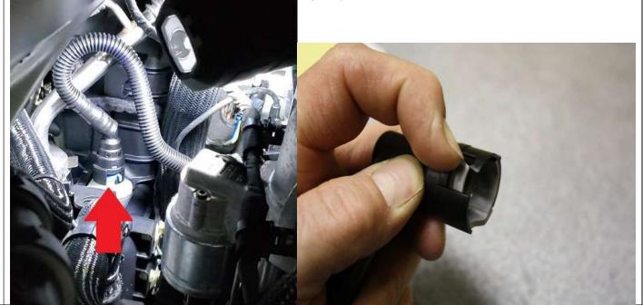
A Now we will need to route the hoses from the top of the vehicle down towards the connections under the engine. We recommend using a piece of tape on one of the hoses to label it for easy identification later in your install. Route hose with male connection in between the Silver metal EGR pipe and intake manifold. Feed hose downward so it's easy to access under the vehicle.
