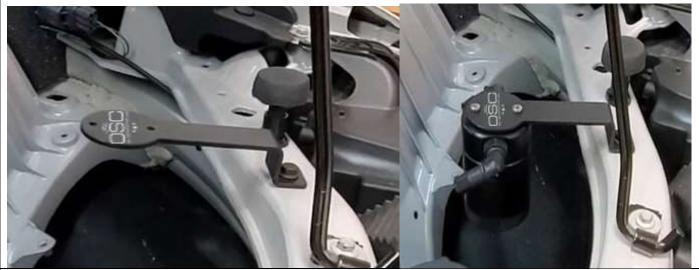
7 The can has a filter installed on the "C" side; this is the dirty side of the can. This needs to connect to the hose that had the MALE fitting. Using light oil, lubricate the inside of the hose and fitting. Install dress up end on hose and push onto the fitting on the "C" side of the can.
