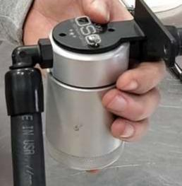
Back at the vehicle, slide threaded clip over preexisting hole on the cowl. Install J&L Separator with J&L supplied bolt. Connect lines back into connections on engine, they will snap into place.
