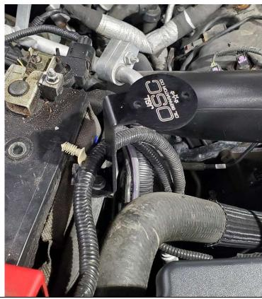
Move J&L Oil Separator into place by routing lining up logos on the oil separator and bracket, slide hose on "C" of the can between the A/C line and battery box. Mount J&L Oil Separator assembly to mounting bracket with the supplied screws, tighten screws.
