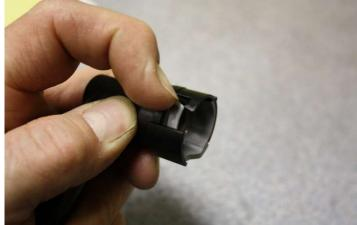
**5** Pry up on push pin in battery box, slide thread clip over exposed hole.
