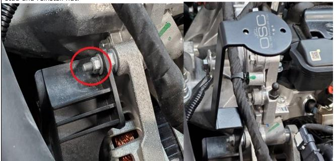
4 Mount J&L Oil Separator to mounting bracket with supplied mounting screws
