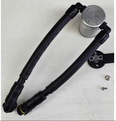
Back at the car, remove small wiring harness clip from stud, you will need to wiggle this off to release. Install J&L Bracket onto stud with J&L supplied nut, tighten nut & reinstall clip. Connect lines back into connections on engine, they will snap into place.
