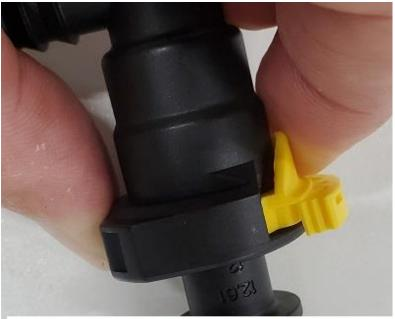
Tab Unlocked, Button pressed to release
