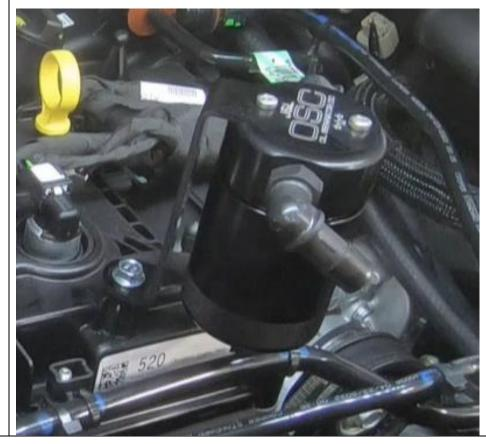
Route J&L hose with the male fitting from the factory line under hard breather line at the front of the engine towards the radiator. You will need to trim this hose to fit, typical trim is 6" off the end of the hose.
