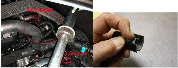
You will need to remove the connection to the intake manifold. Slide the locking tab with your finger and pull fitting away from manifold. Pull hose downward to gain access to the connection.
