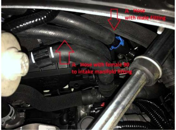
Ensure the hoses are not interfering with the steering shaft, they should be far away from this area. Use zip ties if needed to tie up hoses for extra security.
