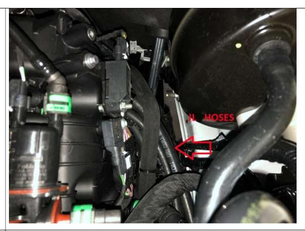
Back under the vehicle, connect J&L 90° fitting to intake manifold. Once the fitting is fully seated you will press in the large tab to lock fitting in. You will hear an audible "CLICK" when it engages. Pull on connector to make sure it doesn't come back off. You cannot see these fittings well, so this is all done by feel.
