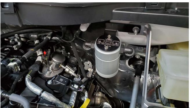
Route hoses around back of engine, run both hoses under the two heater hoses going to firewall. The hose with the 90-degree connection will connect to the PCV valve (valve cover). The hose with the 45-degree connection will connect to the intake manifold.
