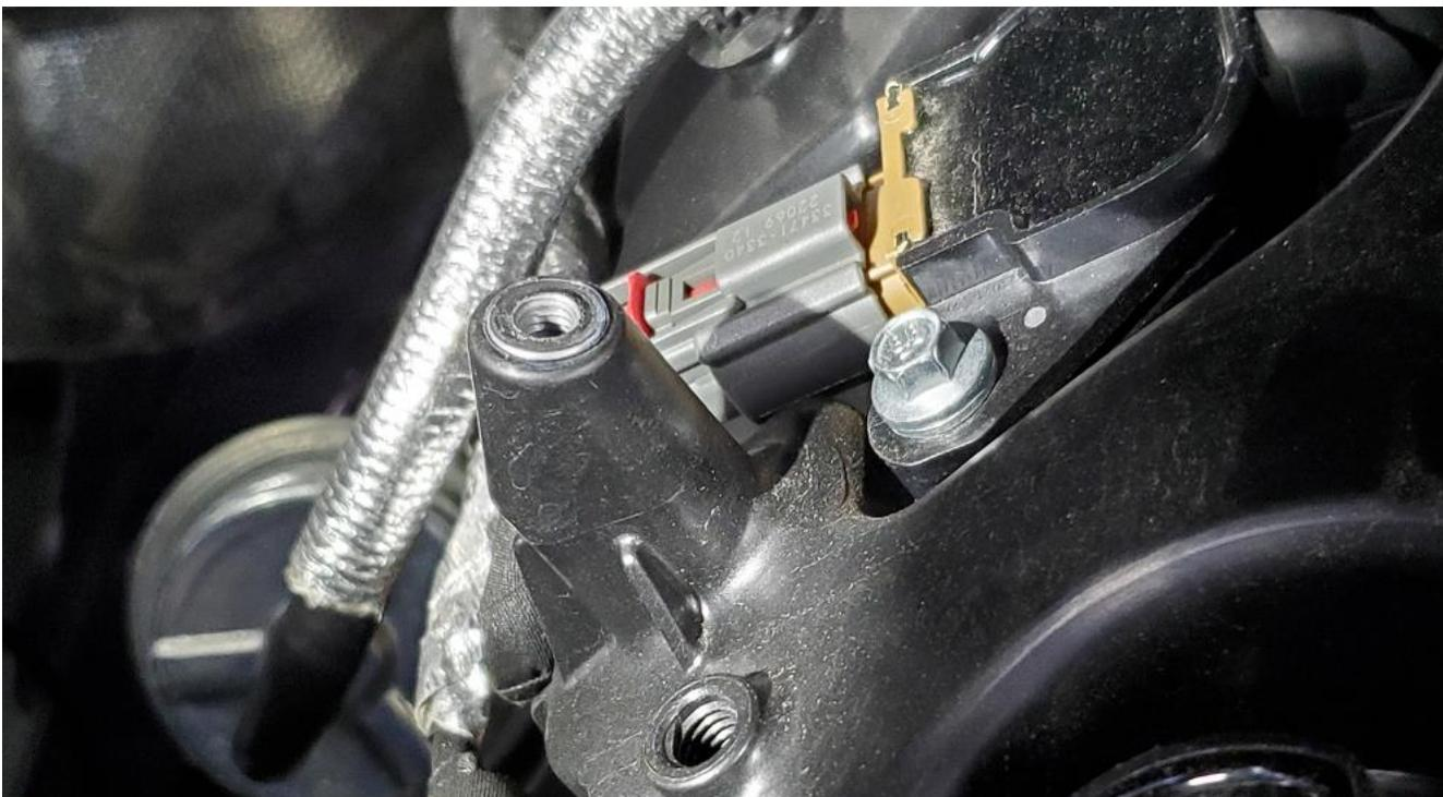
**5** Use supplied screws to mount the bracket onto the Oil Separator, align logos so they match the same direction.
