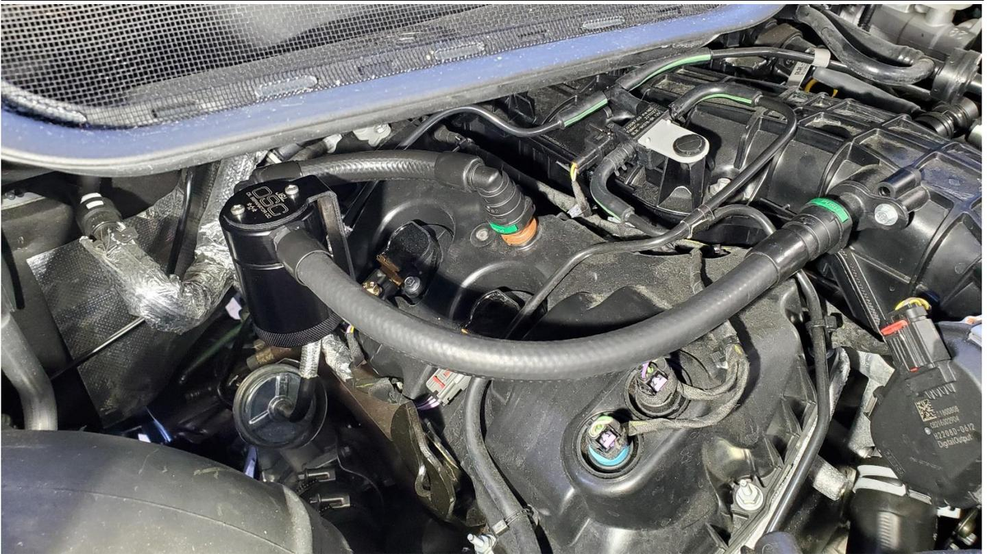
To properly clean the filter in the Oil Separator, spray any degreaser or solvent through it and let it air dry. Clean it every 10,000 miles.
