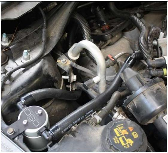
Route front hose through A/C line and connect to the fitting on the manifold and route the rear hose around the back and connect to the fitting on the PCV valve cover.
