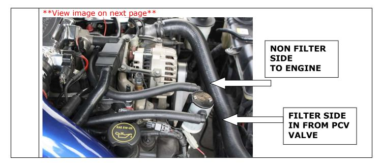
To properly clean the filter in the Oil Separator, spray any degreaser or solvent through it and let it air dry. Clean it every 10,000 miles.
