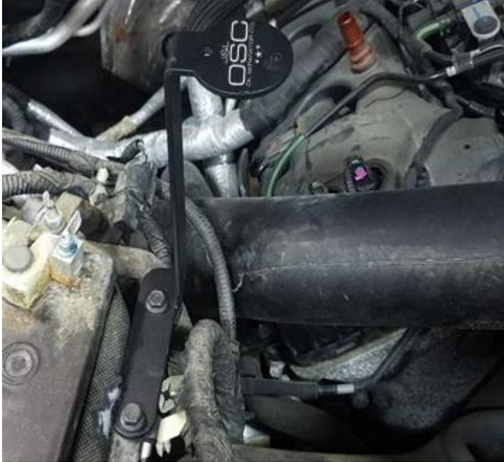
**2021+** - Remove the wire harness tab on the battery tray. Install one of the supplied bolts and nuts through this hole. Using the bracket as a guide mark the 2<sup>nd</sup> hole and drill (optional but recommended) and use the 2<sup>nd</sup> Nut and bolt to secure the bracket.
