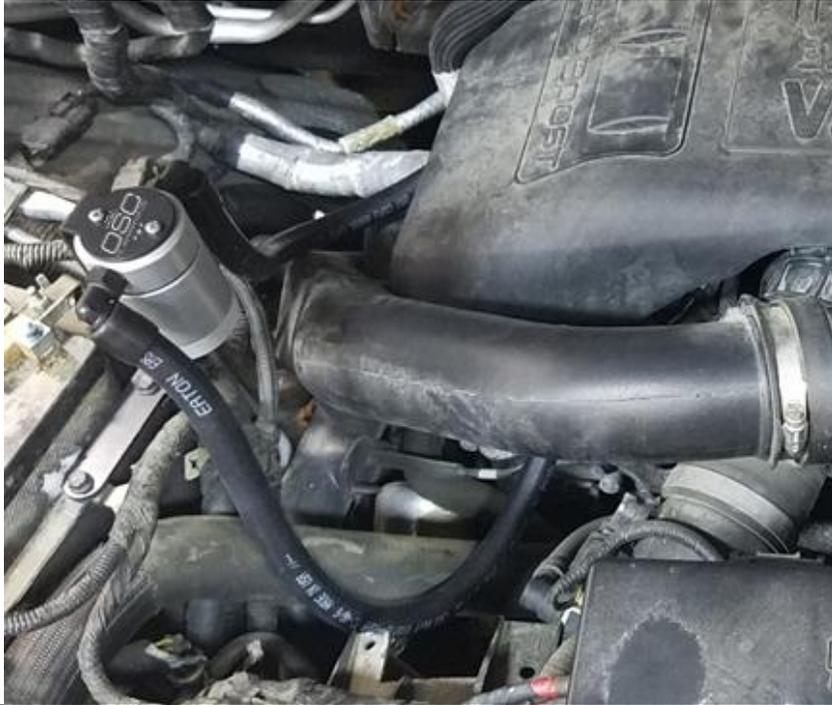
To properly clean the filter in the Oil Separator, spray any degreaser or solvent through it and let it air dry. Clean it every 10,000 miles.
