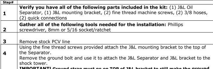
IMPORTANT! Ground strap must go on TOP of J&L bracket to still make the ground.
