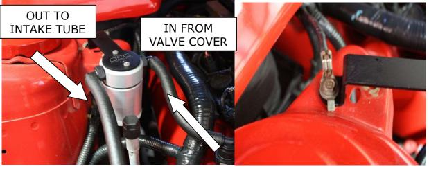
Using the short 3/8 hose, insert the 90° quick connect fitting and to go from the valve cover to the "C" side fitting on the Separator and the long 3/8 hose to go from the front most fitting "O" to the intake tube.
