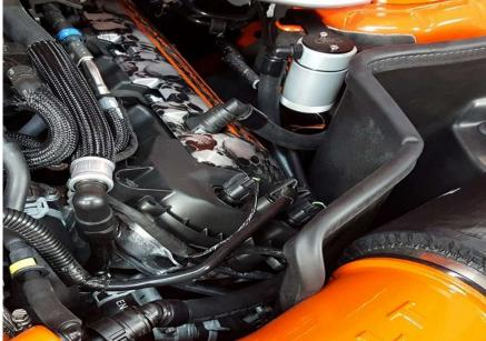
Mount Oil Separator to J&L Bracket with the two supplied machine screws. The longer hose will be closest to the valve cover. Route short hose to valve cover and route long hose to the intake tube.
